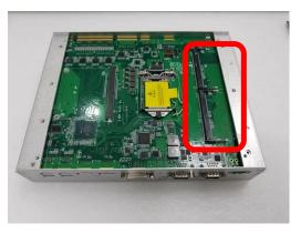
Step 4 Locate the memory module, insert a gold colored contact into the socket and push the module down until it is locked in place by the two end latches.
