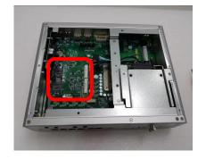
Step 4 Assemble I/O cable to fix the I/O bracket then fasten dual screws of the Flexible I/O Window.
