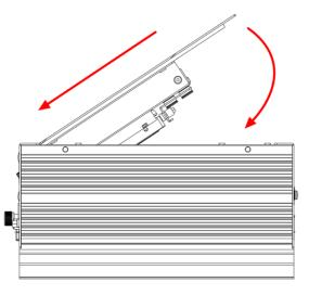
Step 9 Slide the SATA trays back and fasten screws firmly to complete the installation.
