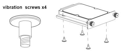
Step 4 Slide the secured SATA drive tray back into the system and fasten the screws firmly to complete the installation.
