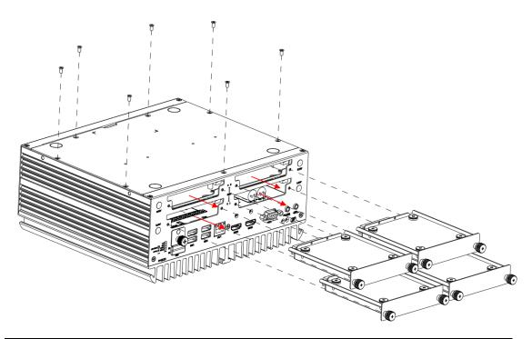
Step 4 Loosen all screws and open the bottom cover carefully.
