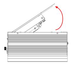
\* After lifting up the cover, please remove the fixed SATA cable first and then put the cover aside.
