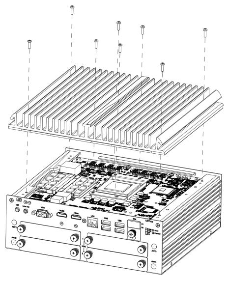
Note: When removing the top cover to change components, the CPU will stick on the underside of the cover. To avoid damaging the CPU by squeezing, please take it down carefully by holding the edges of the CPU and follow section 2.1 to reinstall.
