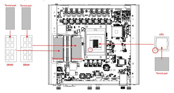
*※* The memory module is locked by two latches on the sides. We recommend using "LDC737" silicone on both sides of the memory for optimal protection against vibration.
