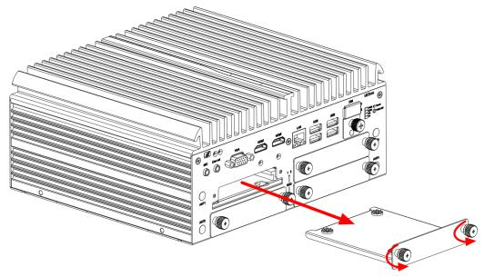
Step 3 Turn the SATA drive tray upside down to install SSD/HDD and fasten the four vibration screws to secure the SSD/HDD firmly to the SATA drive tray.
