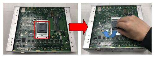
Step 5 Stick thermal pad and install DRAM and CPU.
